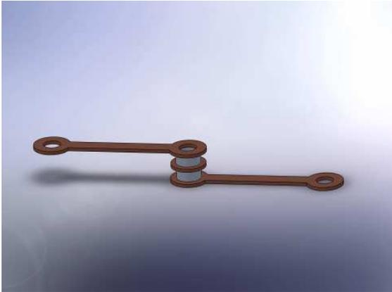
through the traces, or breaking the plating of the hole-barrel will disconnect the endpoints from each other and will therefore be discoverable by testing only the two endpoints. Again, any test probe applied to the via itself will not add significant information.
