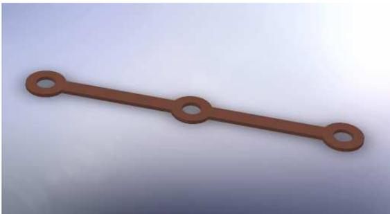
As simple as it is, it makes sense from the standpoint of theory, to examine carefully why it is that we conclude the middle point need not be tested. The middle point need not be contacted because contacting it adds very little information beyond what is already learned by contacting the outer two points. If the trace is “cut anywhere”, then that discontinuity will be discovered when a test is applied to the outer two pads. Of course this is not *completely* true.
