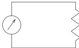
The drawing shows the meter directly connected to the resistance of the device that is being measured. This drawing, although not completely correct, is a close enough approximation when we are measuring the resistance of devices that are MUCH higher than that of the wires connecting the meter to the resistor.
