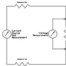
As you can see, the extra two wires allow the voltage across the device to be sensed through separate that carry very low (essentially zero) current. Since there is no current, there is no voltage developed across the leads. The voltage measured by the meter is the actual voltage across the device.
