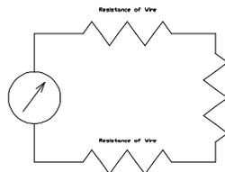
The new drawing shows the resistance of the wires that connect the meter to the device. The current through the resistor is identical to the current through the meter and the wire leads – no problem there. Unfortunately, the voltage measured by the meter is the voltage across the resistor *plus* the voltage
